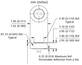
0.03 (0.001) Minimum Ref. (applies to top edge of gasket or edge of crimp, whichever is higher)
